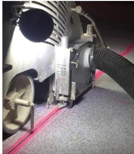
Figure 6 Photo of Early Entry Saw Joint With Vacuum Attachment
