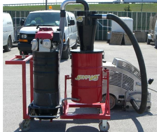
Figure 5 Photo of Early Entry Saw Vacuum Pickup Equipment
