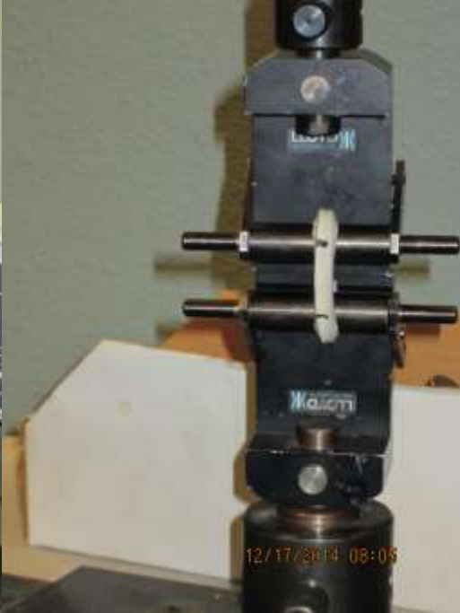
Figure 2 – Before Tensile Test
