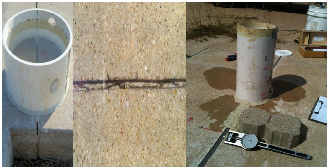
Figure 7 Flow Test on Existing Joint.
