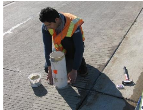
Figure 22 SR 59 Infiltration Testing (2013).
