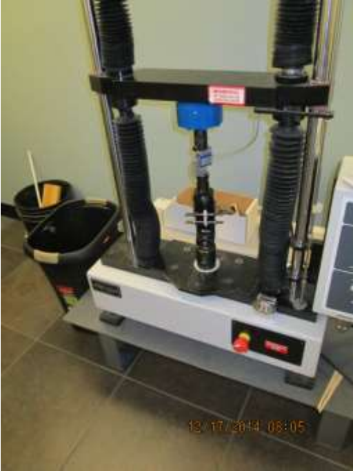
Figure 1 – Tensile Test Set-Up
