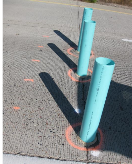
Figure 26 I-10 SPS-2 Infiltration Position 1 (interior), 2, and 3 outer edge Testing.
