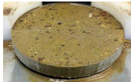
Figure D.1 Erosion Test Using Hamburg Wheel-Tracking Device.
