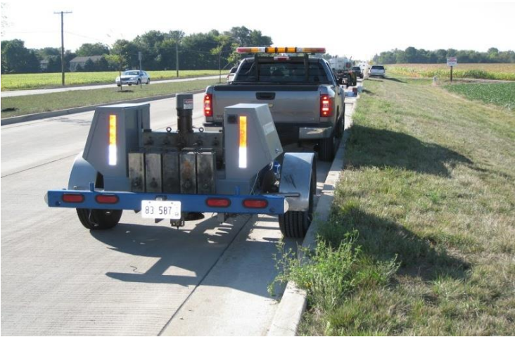
Figure 23 SR 59 FWD Testing.
