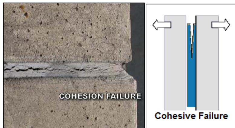
Figure 2 Cohesive Failure in Sealants.
