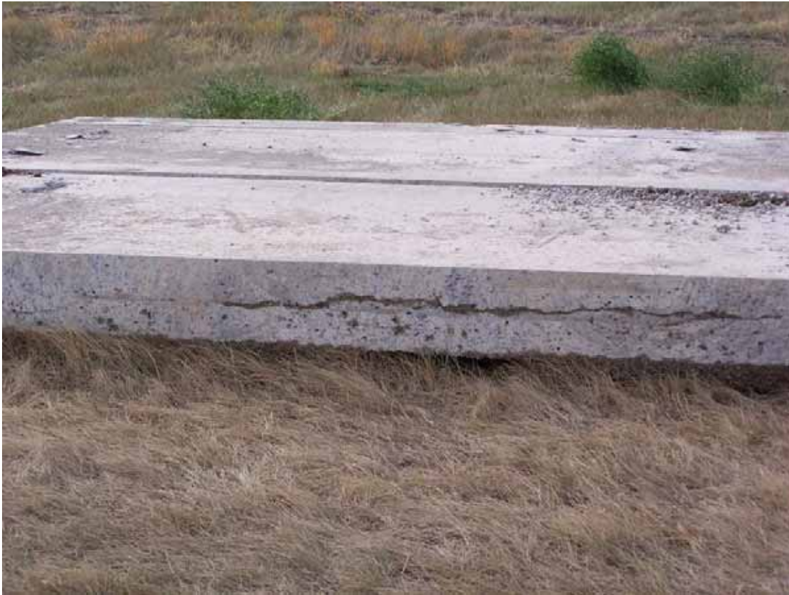
Photo 25 – Photo of crack running transversely in the center of a pavement section removed from roadway.
