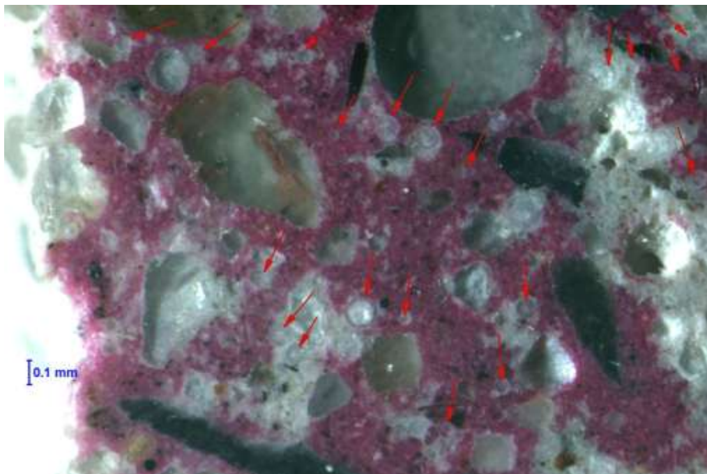
Photo 4: Translucent secondary ettringite fills most entrained air voids directly adjacent to a vertically spalled joint surface (L). Paste was stained magenta with phenolphthalein to aid in identifying filled voids.
