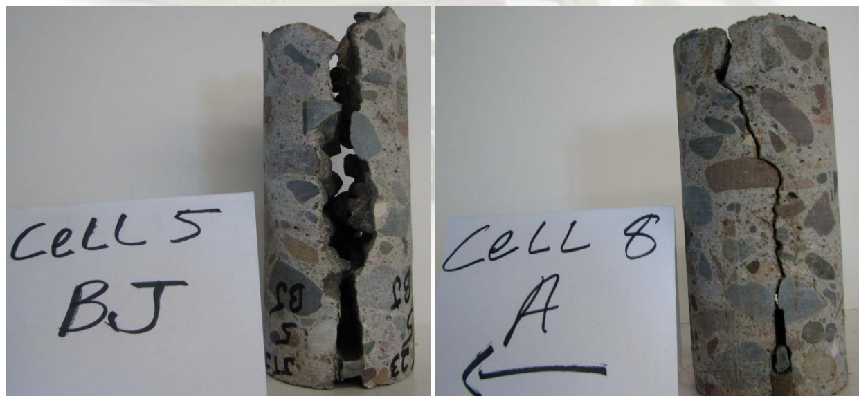
Photo 1. A) Core sample “BJ” (shown inverted) from joint over nondrained gravel base. B) Sample “A” from joint over drainable PASB.
